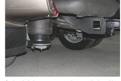
Optional air-bag rear suspension was designed by Accubuilt and replaces stock leaf springs.
