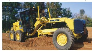
converter and use the machine in a direct-drive mode with an inching pedal. According to Komatsu, the torque-converter mode, available in the four lower gears, provides increased tractive effort and finer low-speed control.
