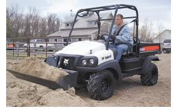
as high as 2 feet, and when not required, the system can be removed for conventional operation of the vehicle. The 2300 features a 20-hp diesel engine, as well as the Bobcat IntelliTrak drive system. It can haul 800 pounds in its power-dump cargo box.
