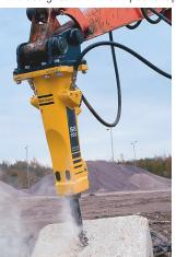
fined spaces. New in the line are the 183-pound SB 100 and 275-pound SB 150, designed for use on smaller carriers. Maximum impact frequency is 2,280 blows per minute, and both new breakers operate in a pressure range of 1,450 to 2,175 psi. The SB 100 requires an oil flow of 4.2 to 9.2 gpm, and the SB 150 requires 6.6 to 10.6 gpm.
