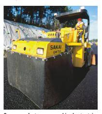
Some manufacturers are making heat-retaining skirts standard equipment on pneumatic rollers to discourage asphalt pickup.
