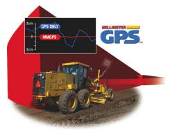
The LazerZone™ transmitter blankets an area over 30 feet tall and up to 2000 feet in diameter with vertical precision. Up to four transmitters can be linked for wide / tall area coverage. An unlimited number of Topcon 3D and RTK GPS rovers can be equipped to receive the LazerZone signal.
